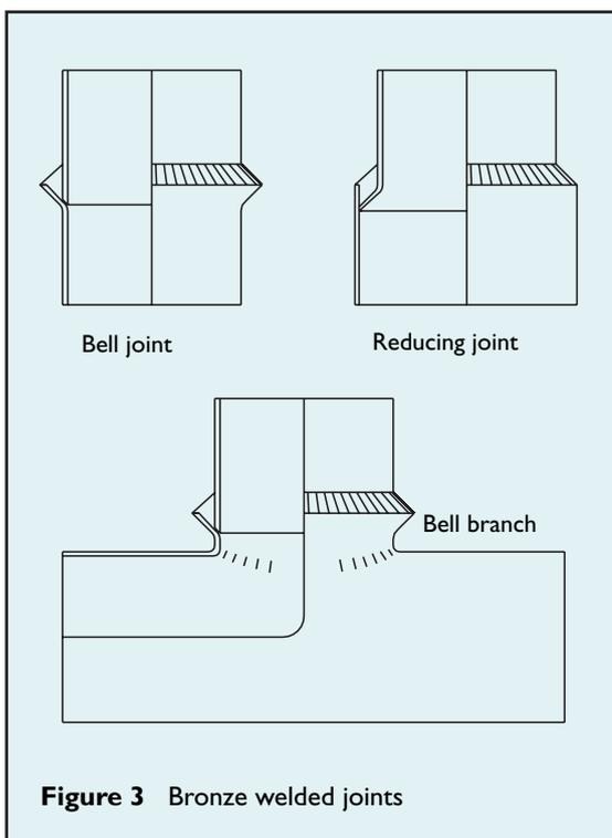
**Figure 3** Bronze welded joints
