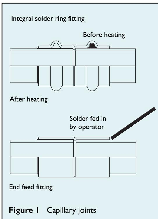
**Figure 1** Capillary joints
