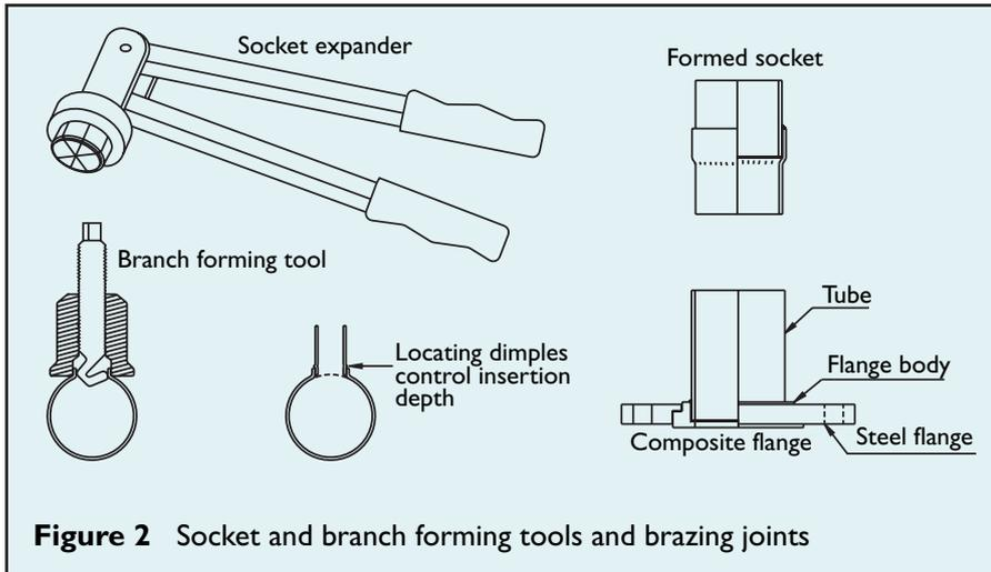
**Figure 2** Socket and branch forming tools and brazing joints
