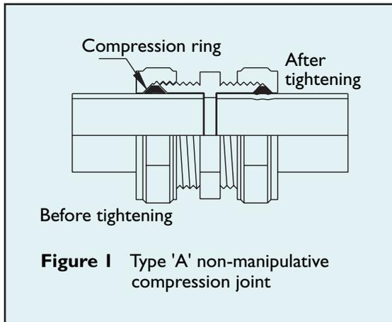
**Figure 1** Type 'A' non-manipulative compression joint
