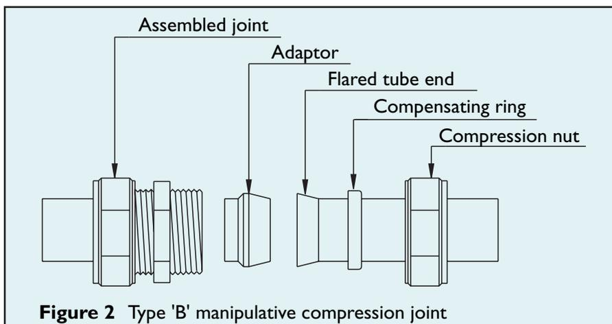
**Figure 2** Type 'B' manipulative compression joint
