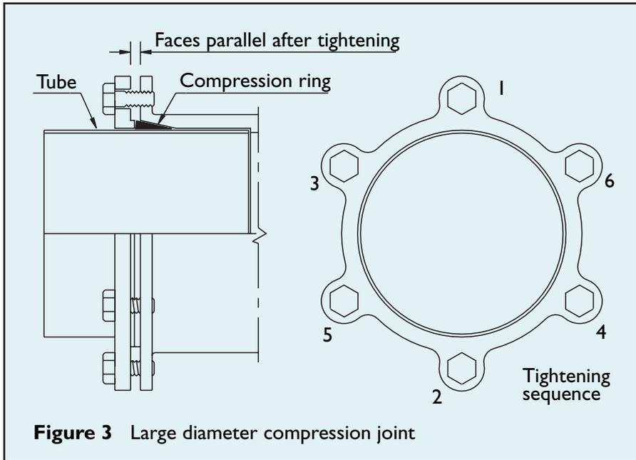
**Figure 3** Large diameter compression joint
