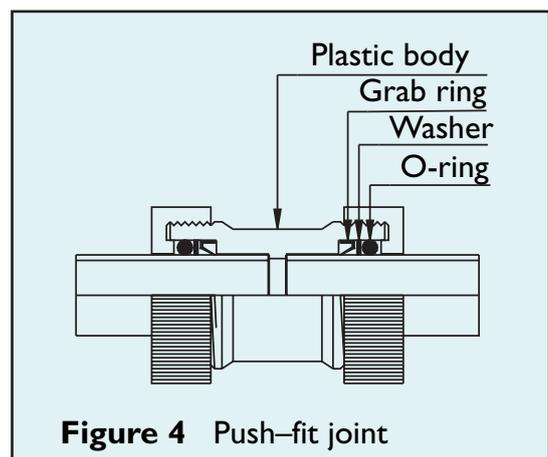
**Figure 4** Push-fit joint
