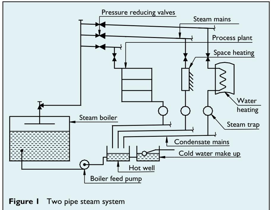
Figure 1 Two pipe steam system
