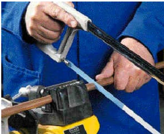
*Figure 4 – Cutting tube*
